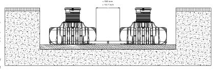
GARANTIA special crown bit. It must be ensured that the distance between the tanks is at least 500 mm (19.7 inch). The pipes must project at least 200 mm (7.9 inch) into the tanks.
