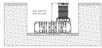
Allowed earth coverage height with GARANTIA extension riser and passenger car module with cast iron cover (class B) in areas used by passenger cars (max. total load 3.5 ton).
